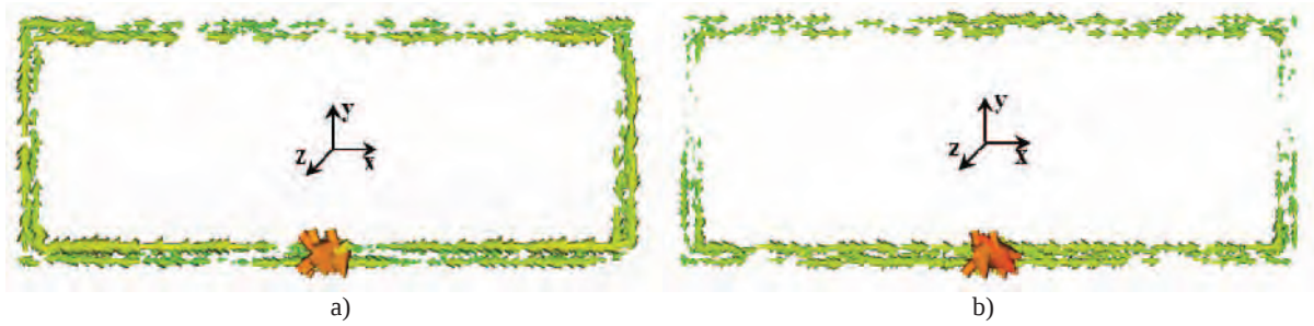
Fig. 4. Current distribution at the frequency 870 MHz along (a) the loop with SRRs , (b) the conventional loop.
